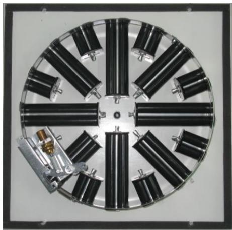
The automatic adjustment of the blades angle is succeeded with a thermal actuator which according to the supply air temperature moves an axis. This movement is very intensive between 20-28°C, outside this temperature area the movement very small.
