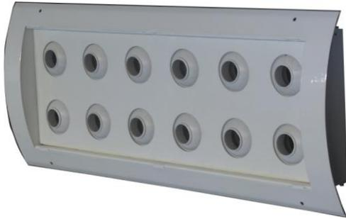
The jet diffusers AMB-AP-SR series have a curved frame manufactured by galvanized steel sheet or steel sheet electrostatically painted in RAL color, which allow them to be installed in the side of visible round air ducts. They are manufactured with a curvature same as the air duct curvature, so a perfect fit and a high design are achieved.
